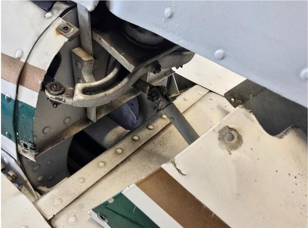
You can actually place the 10 lb ABW into the tail without fully removing the tail cone cover, but the cover really needs to be removed, when you use a drill.
