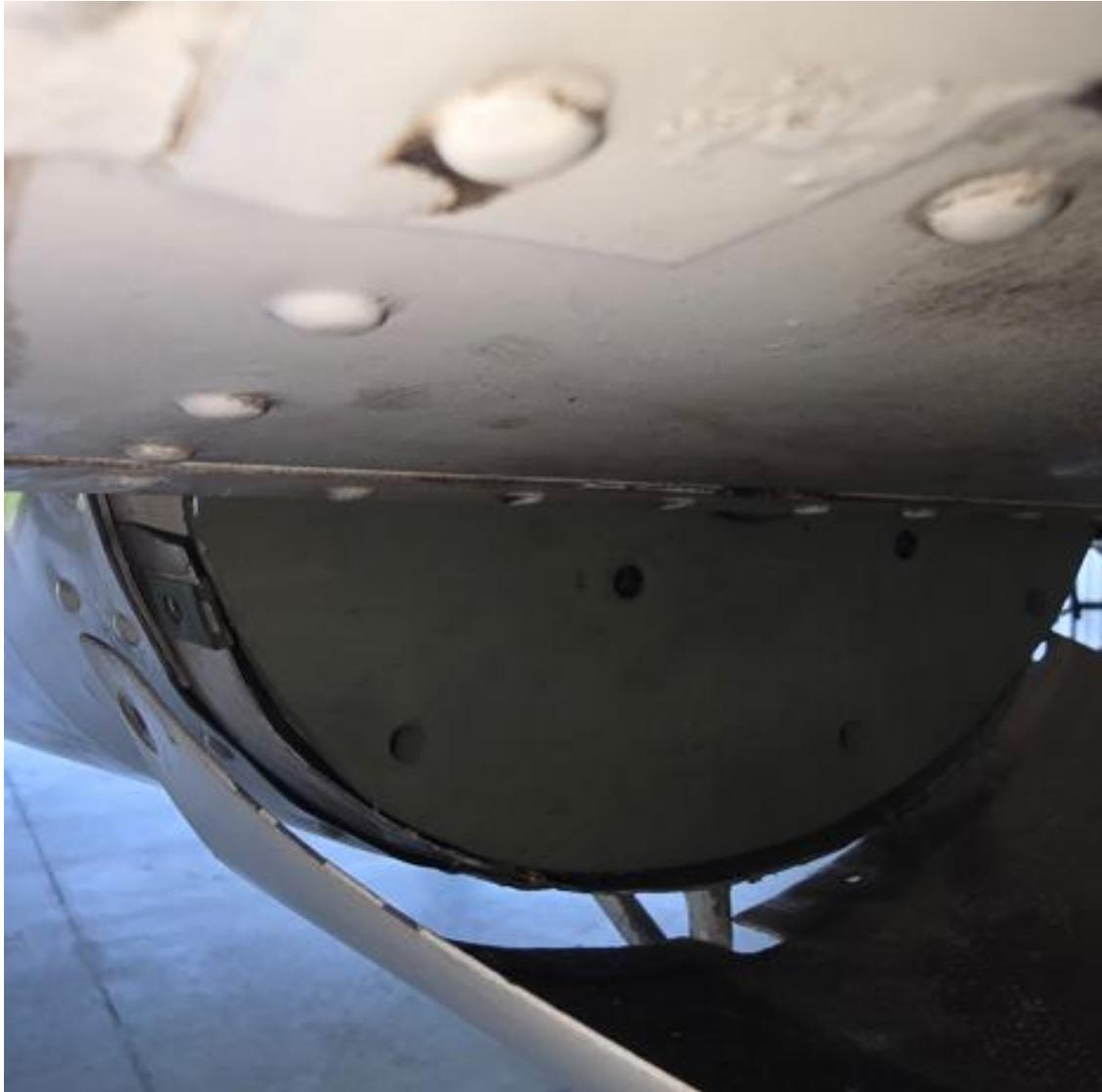
The 10 pound ABW is just rested in place, at its prescribed location at station 288. At different stages of the installation it is a good idea to check the horizontal stabilizer counterweight arm clears all of the new components, and check that the horizontal stabilizer does not contact anything on the ABWs including the hardware. No issues were observed on this particular installation.
