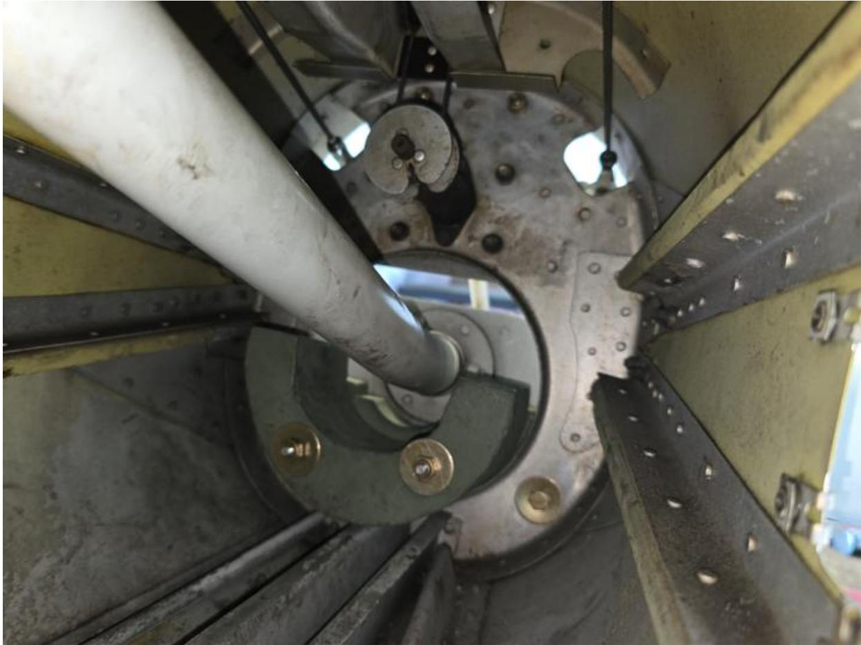
The two nuts for the supplemental weight are installed thru the access panel and the **22 ABW is installed at this point**, and then the removable panels are reinstalled. A magnetic pick up tool might be handy if a nut or washer was to fall into the series of aluminum channels running along the bottom of the tail.
