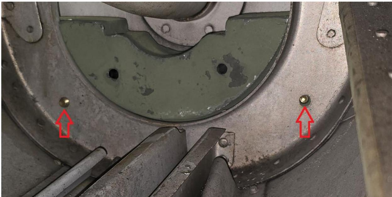
The holes lined up very close on the right side, but after temporary installing the nut on the left, then the right bolt was removed and the hole was "cleaned up" with a  $\frac{1}{8}$ " drill bit and the right bolt was installed.
