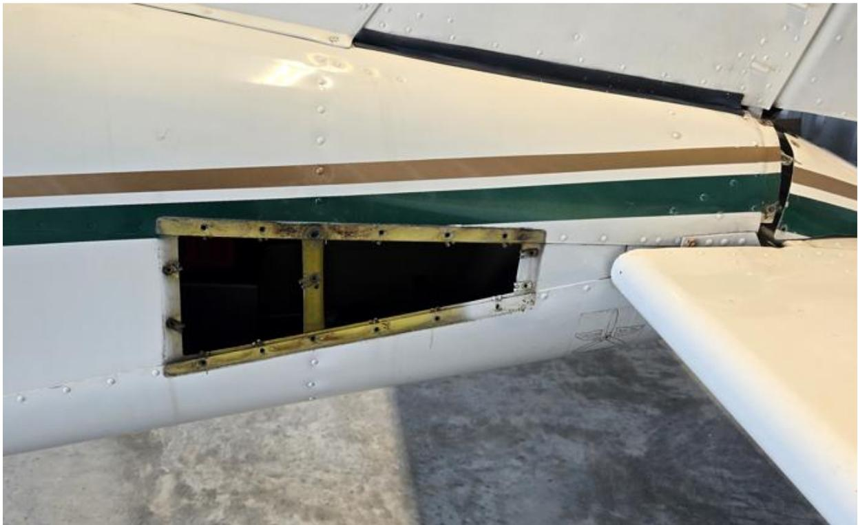
I loosened the fiberglass tail cone cover, and disconnected the arm that is attached to the horizontal stabilizer trim. I never removed this part previously but with a little manipulation it comes right out. You
