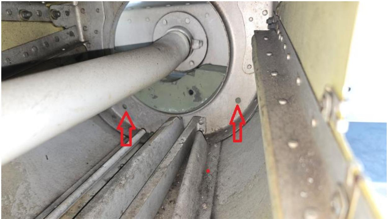
Looking inside of the tail thru the access panel you can see the two tooling holes that are used to bolt the 10# assembly to the aircraft frame.
